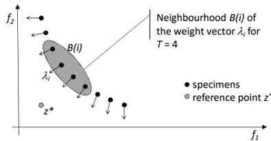
Fig. 1. An overview of concepts involved in the working of the MOEA/D algorithm in the case of minimization in a bi-objective problem.
